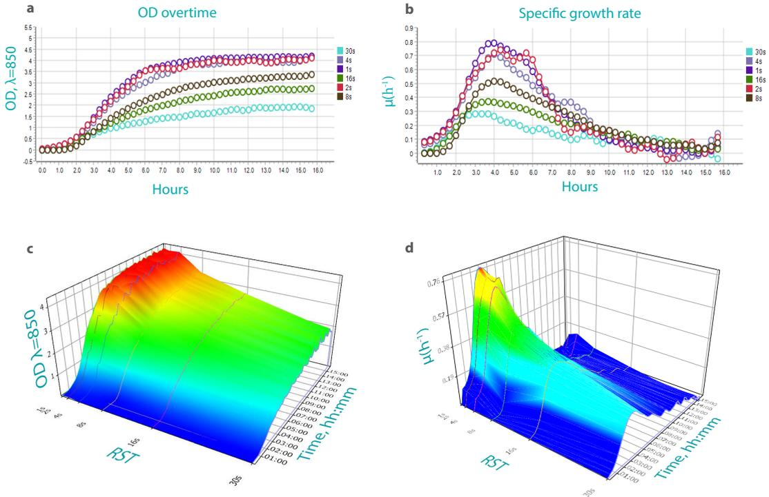
Figure 2, a-c. Influence of Reverse Spin Time (RST) on growth kinetics of *E. coli* BL21 in  $OD_{850}$ . (a-c) Biomass growth; (b-d) Specific growth rate; throughout cultures were grown in 50 ml TPP Bioreaktor tubes, 30% filling volume, 2000 RPM, RST 1, 2, 4, 8, 16, 30 seconds, LB medium and 37 °C temperature, to convert  $OD_{850}$  to  $OD_{600}$  simply multiply  $OD_{850}$  by 1.9.
