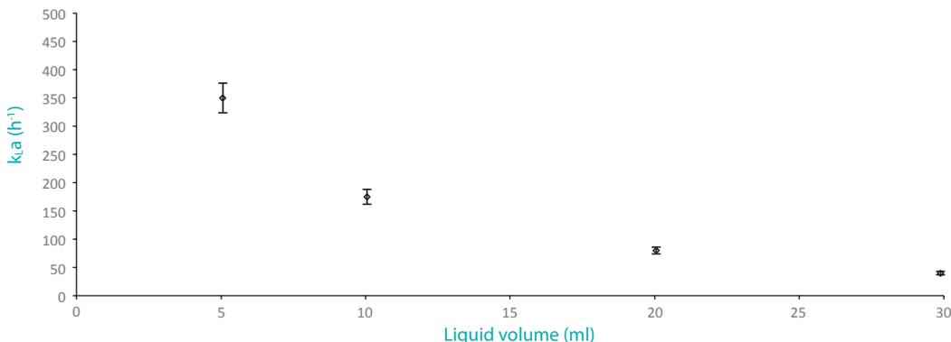
Figure 3. Determination of  $k_La$  in 50 ml TPP Bioreaktor tubes. The bioreactor vessels were filled with 5, 10, 20, 30 ml deionized water, and measurements were made by non-invasive  $O_2$  sensors and optics (PreSens, Regensburg, Germany) at 37 °C using the gassing-out method. Mean and standard deviation of at least five independent experiments are shown.
