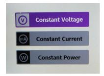
2. Use the up and down arrows to select which parameter should be kept constant. Press the enter key to move to the next page.
