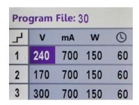
7. Pressing the pause key will temporarily pause the run and will allow parameter values to be altered using the same method outlined above.
